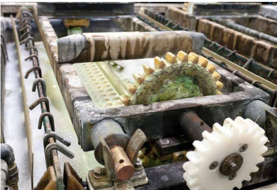
**Fig. 2:** Release of hydrogen and foam building up in electrolytic degreasing operations. The workpieces are usually immersed into an alkaline solution containing tensides and are connected either to the anode or the cathode. The current densities of up to 15 A/dm<sup>2</sup> applied here cause violent hydrogen and oxygen development. The tiny gas bubbles rising from the workpiece surface remove the remaining lubricating oil and grease particularly thoroughly.
