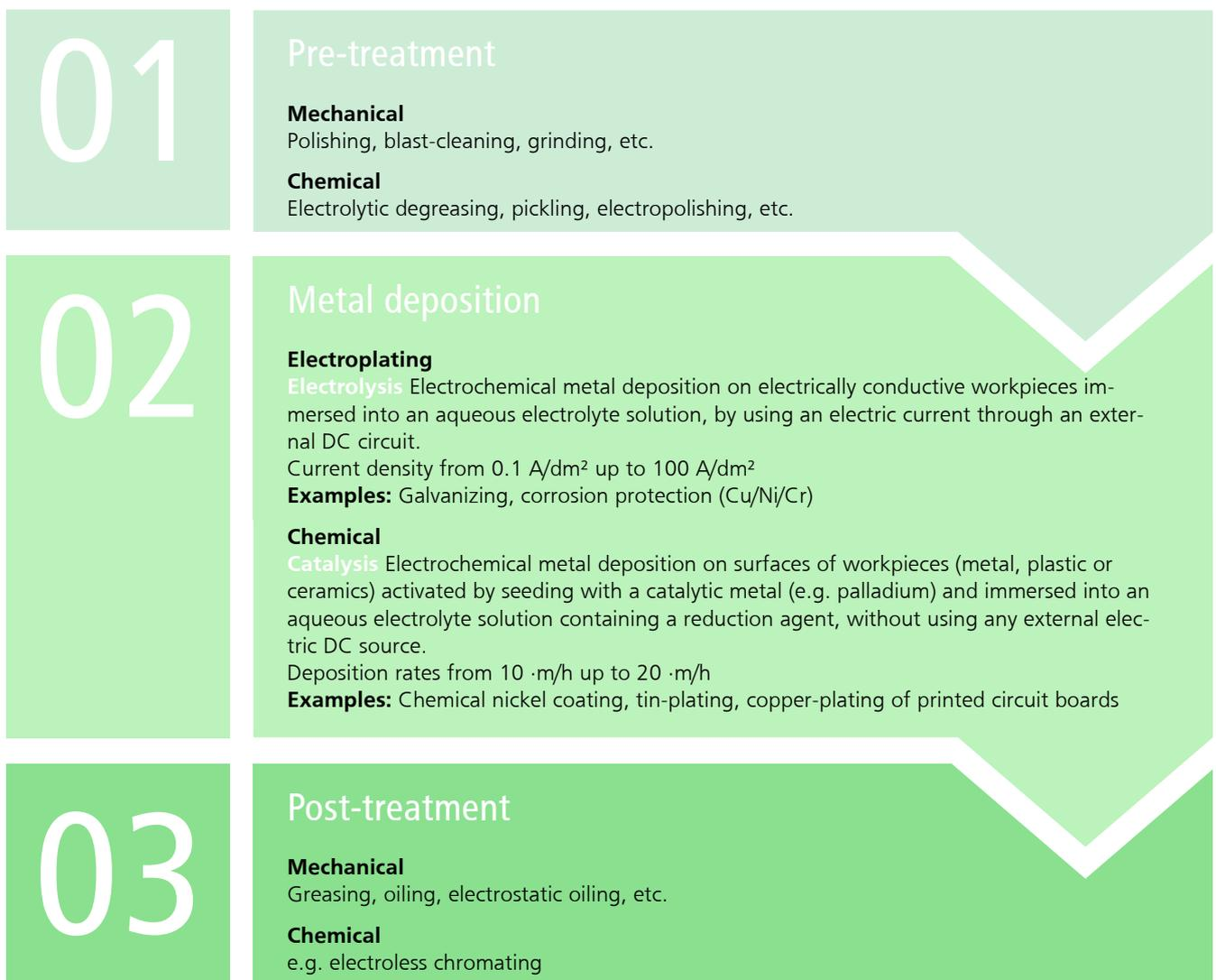
**Fig. 4:** Fundamental process steps of electroplating process
