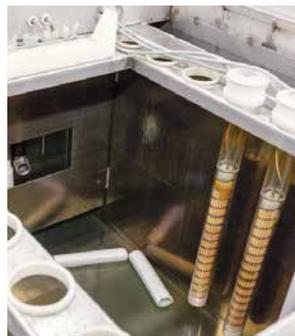
**Fig. 7a:** Heating elements with thermal discolorations of heating cartridges and electric cables.
