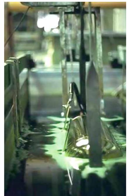
**Fig. 3:** Electropolishing of a workpiece while releasing hydrogen. This method is used predominantly above all for levelling stainless steel surfaces. After immersing in strong acids, the workpieces are connected as an anode and metal out-of-flatness in the micrometer range is removed by electrochemical means so that a smooth and shiny surface is obtained. Current densities of up to 100 A/dm<sup>2</sup> are employed here.
